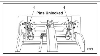
Figure 3-20 Attachment Locks in Unlocked Position
